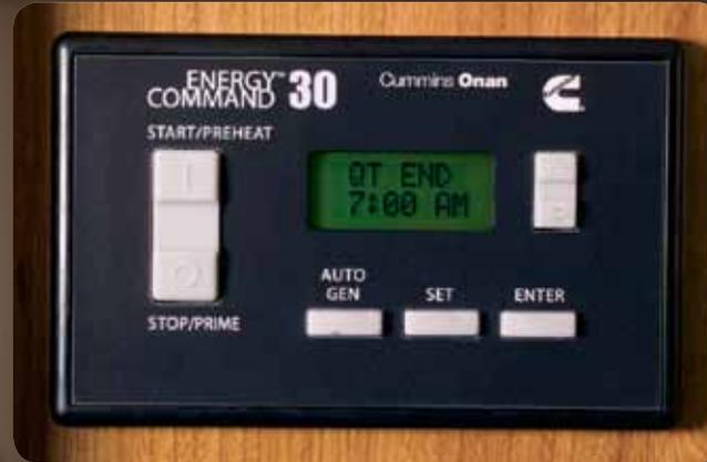
**Auto Start** The available automatic generator start system automatically starts the generator to charge the system when the coach batteries run low and can also be programmed to turn on at a pre-set time or temperature so you can return to a cool coach.
