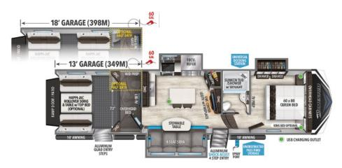
349**M** UVW HITCH<sup>†</sup> GWVR LENGTH! HEIGHT CAPACITY 13'5" 2,925 17,000 38' 11" 155 104 52 13' GARAGE 13,600 398M UVW HITCH GWVR LENGTH: HEIGHT CAPACITY 15,000 2,980 20,000 155 104 52 43' 11" 13'5" 18' GARAGE
