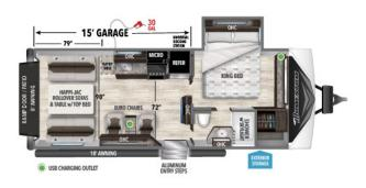
EMPTY HITCH 23**G** UVW GVWR CAPACITY LENGTH<sup>‡</sup> HEIGHT 15' GARAGE 6,897 1,266 13,000 28'10" 12'4" 100 74 39
