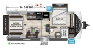
EMPTY HITCH 21**G** UVW **GVWR** LENGTH1 CAPACITY HEIGHT 6,400 920 11,000 26' 11" 12' 2" 100 74 39 14' GARAGE
