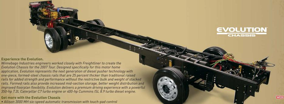
• I-beam axle with a 55-degree wheel cut
