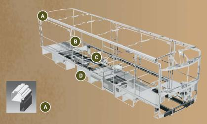
SUPERSTRUCTURE® is the term given to Winnebago Industries' structural motor home design and construction. Rather than a single component, it is the culmination of design integration that incorporates steel and aluminum substructures; welded tubular steel floor risers; interlocking joint technology; and Thermo-Panel® floor, roof and sidewalls to form a high-strength, durable vehicle body.
