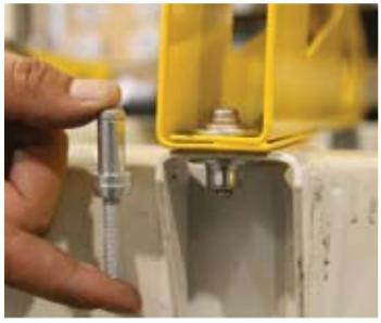
Huck fasteners can't be over or under tightened ensuring the strongest and longest lasting connection of the truss system to the chassis.
