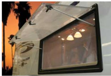
The outer pane is mounted awning style to keep light rain out and still allow the fresh air in.
