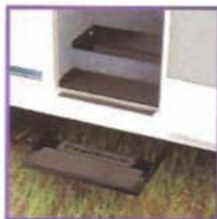
▲ Step wells feature rubber step treads, and a rare class C option: An electric entrance step with a dash warning light.
