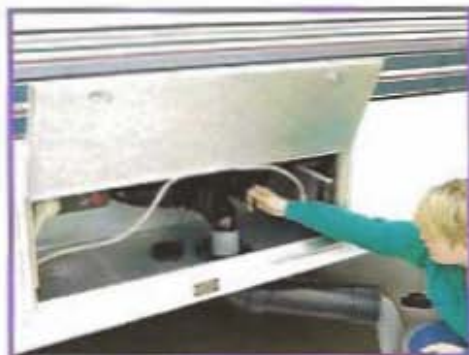
▲ Your hose stores in the convenient swiveling boom, allowing you to leave the hose connected to your system. With the boom you can easily position the hose with a minimum of handling.
