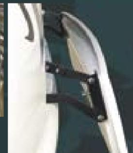
**Pantographic hood hinges** and "finished" backside of hood speak to National RV's attention to quality and detail even in seldom-seen areas of the coach.
