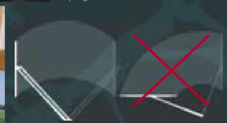
**Pantographic windshield wipers** (left) clean a wider swath of windshield than typical radial windshield wipers (right) of similar blade length.
