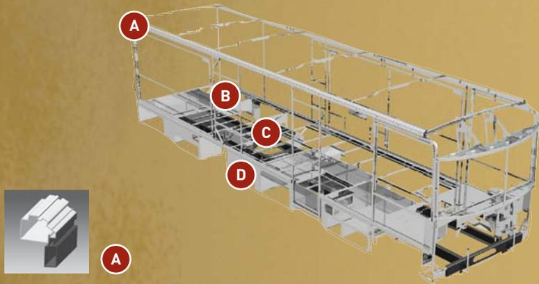
**SUPERSTRUCTURE®** is the term given to Winnebago Industries' structural motor home design and construction. Rather than a single component, it is the culmination of design integration that incorporates steel and aluminum substructures; welded tubular steel floor risers; interlocking joint technology; and Thermo-Panel® floor, roof and sidewalls to form a high-strength, durable vehicle body.
